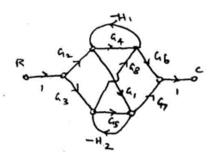
12. Considering the system shown in figure, obtain the transfer function using Masons Gain formula.
