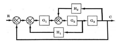
8. Using block diagram reduction rules, obtain the closed loop transfer function C(S)/R(S) of the given
