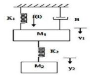
**10.** For the given rotational mechanical system, write the differential equations and find the transfer system function
