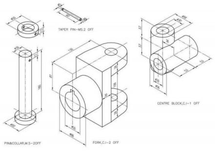
Note: Print the orthographic view and sectional view from the above assembled 3D drawing.
