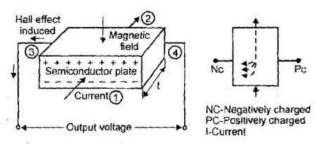
Current is passed through leads 1 and 2 of the semiconductor plate and the output leads are connected to the element faces 3 and 4.
