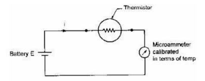
The thermistor is an extremely sensitive device because its resistance changes rapidly with temperature.
