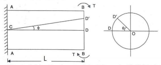
When the shaft is subjected to torque T then D is moved to  $D^I$ . If ' $\phi$ ' be the shear strain and ' $\theta$ ' be the angle of twist in length I then
