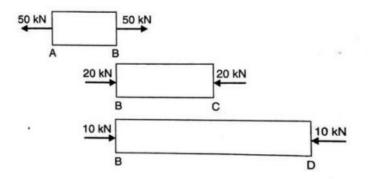
**Part AB.** This part is subjected to a tensile load of 50KN. Hence there will be increase in length of this part.
