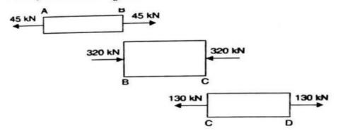
From Fig it is clear that part AB is subjected to a tensile load of 45 kN, Part BC is subjected to a compressive load of 320 kN and part CD is subjected to a tensile load of 130kN.
