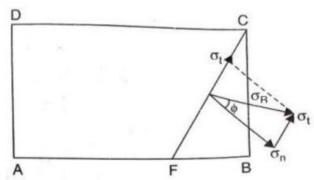
**Maximum Shear stress**. The shear stress is given by  $\sigma_t = \frac{(\sigma_1 - \sigma_2)}{2} \sin 2\theta$ . The shear stress will be maximum when
