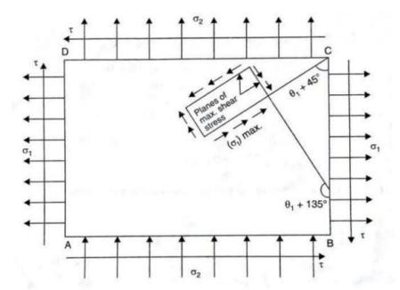
**Problem.1.21.**The tensile stresses at a point across two mutually perpendicular planes are 120N/mm<sup>2</sup> and 60N/mm<sup>2</sup>. Determine the normal, tangential and resultant stresses on a plane inclined at 30° to the axis of minor stress
