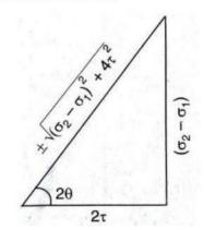
Substituting the values of  $\sin 2\theta$  and  $\cos 2\theta$  in equation (ii), the maximum and minimum shear stresses are obtained.
