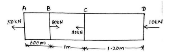
**Given Data:** A = 1000 mm<sup>2</sup>, E =  $1.05 \times 10^5 \text{ N/mm}^2$
