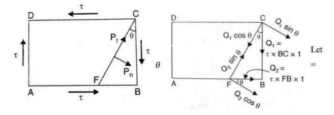
Angle made by oblique section FC with normal cross section BC,
