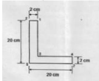
2. Explain the method of determining the free-end deflection of a cantilever beam subject to a tip concentrated moment  $M_0$  in a plane inclined at  $\theta$  to the vertical plane. The beam is uniform with an unsymmetrical cross-section.
