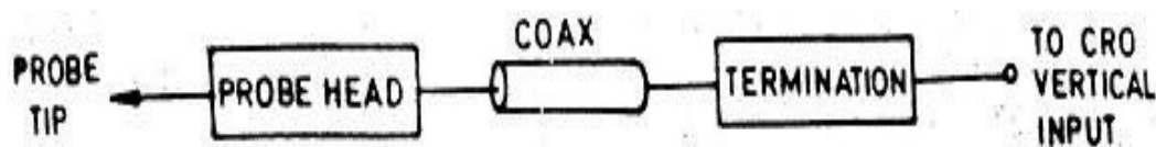
Fig 2.8.1 Block diagram of general purpose probe
