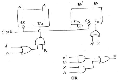
b) (i) Construct a timing chart for the network for an input sequence X=10011. Indicate at what timer Z has the correct value and specify the correct output sequence.(Assume that X changes midway between clock pulses) Initially,  $Q_1=Q_2=0$
