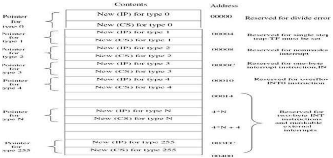
Figure 1.6.1 Organization of Interrupt Vector Table (IVT) in 8086
