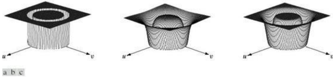
(Fig3.4.1: Perspectives plot of ideal, Butterworth , Gaussian and Notch
