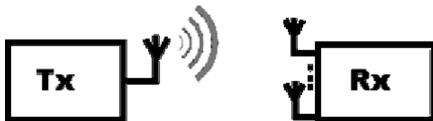
Fig.5.7: SIMO - Single Input Multiple Output
