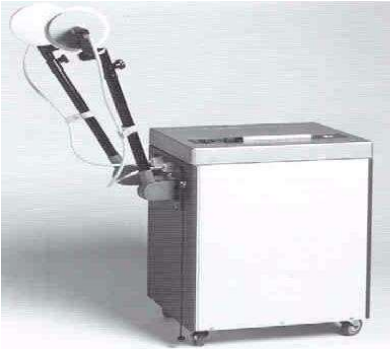
Fig:5.2.2 Short wave diathermy unit
