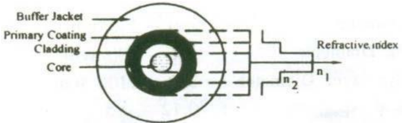
Fig 2.12.1 Single mode fibres
