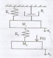
a) Determine the transfer function for the figure shown in below by using block diagram reduction technique.
