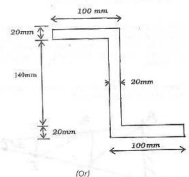
(b) Find the moment of inertia about the centroidal axis XX and YY of the section shown in fig.
