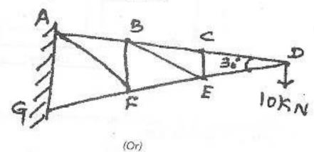
(b) A simply supported truss is loaded as shown in fig. Find the reactions and forces in all the members of the truss by graphical method and indicate whether forces are in tension or compression.
