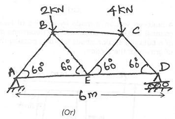
(b) A cantilever truss is shown in fig. Find the forces in all the members of the truss by graphical method and indicate whether forces are in tension or compression.
