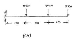
(b) Draw the SFD and BMD for the beam as shown in figure.
