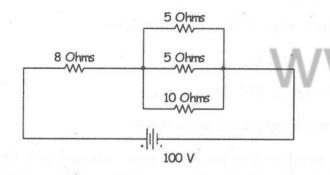
18. (a) By using mesh current analysis, find the current supplied by the batteries.
