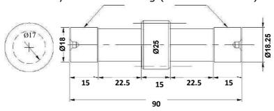
Exercise No: 6- Progressive type Plug gauge (Cylindrical Grinding)
